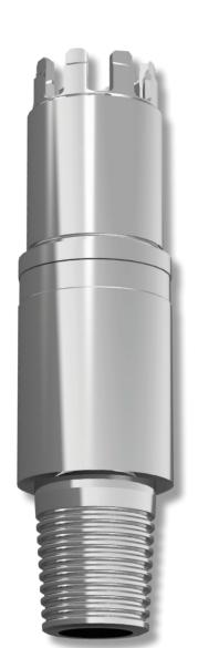
The Cablehead Termination Sub delivers an alternative configuration of the INFOCOIL BHA system, allowing a swift change to conventional coiled tubing operations without removing the Cablehead or TEC Cutter. When installed on the Cablehead, this sub seals the electrical port and adapts to a standard thread for maximum flexibility.
