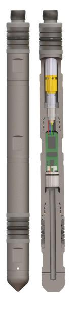
The 1.00" OD Side Pocket Gauge is a dual function Piezo Gauge assembly designed with seal stacks for plugging off an industry-standard 1.00" Side Pocket Mandrel. The gauge is capable of recording internal or annular tubing pressure and temperature accurately.
