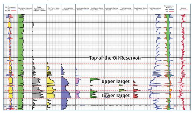
Analysis and interpretation of the horizontal log keeps you in the zone of interest and can differentiate between tight, fractured, or more porous zones.
