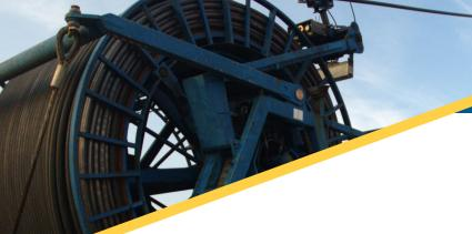
Reservoir Group introduces the INFOCOIL System which is capable of providing real-time data during well intervention operations. The system is highly beneficial for ultimate job performance and success by delivering "live" downhole internal and external pressures, tension / compression, and temperature data along with a casing collar locator (CCL) for accurate depth control. The system includes a surface equipment package, downhole tools, and 1/8" Tubing Encapsulated Cable (TEC).
