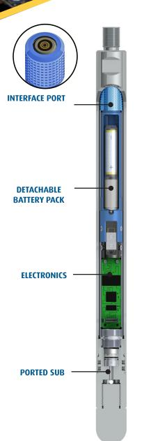
Reservoir Group's Apex gauge excels in remote operations - fully automated, Apex requires no operator input to accurately record downhole pressures and temperatures.
